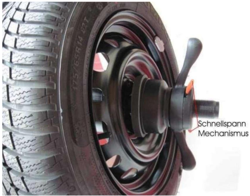
Fig. 9 Removing the wheel from the bracket.
