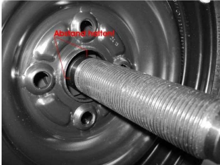
Fig. 8 Mounting a car wheel in the bracket
